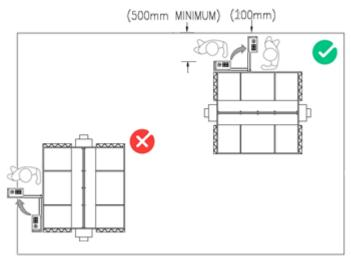
d) Access panels to machinery exhibits should be positioned to ensure that when the door is fully open it remains within the stand boundary:
