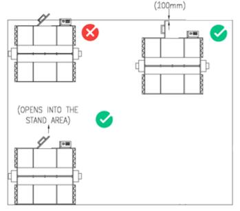
e) **OPERATING PLATFORMS** - Operating platforms around individual exhibits or parts thereof may be permitted but must be suitably enclosed to conform to Health and Safety regulations. Also, a sign must indicate that 'Machine Operators Only' clearly displayed.
