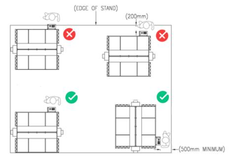
i) Static operating panels facing the aisle must be set back 500mm:
